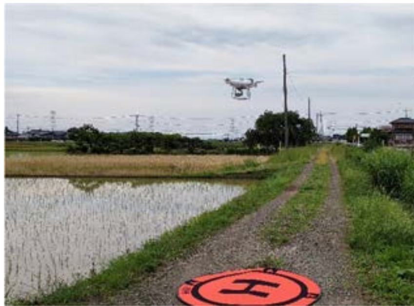
Figure 4. P4 Multispectral camera-mounted UAV used in the study.
