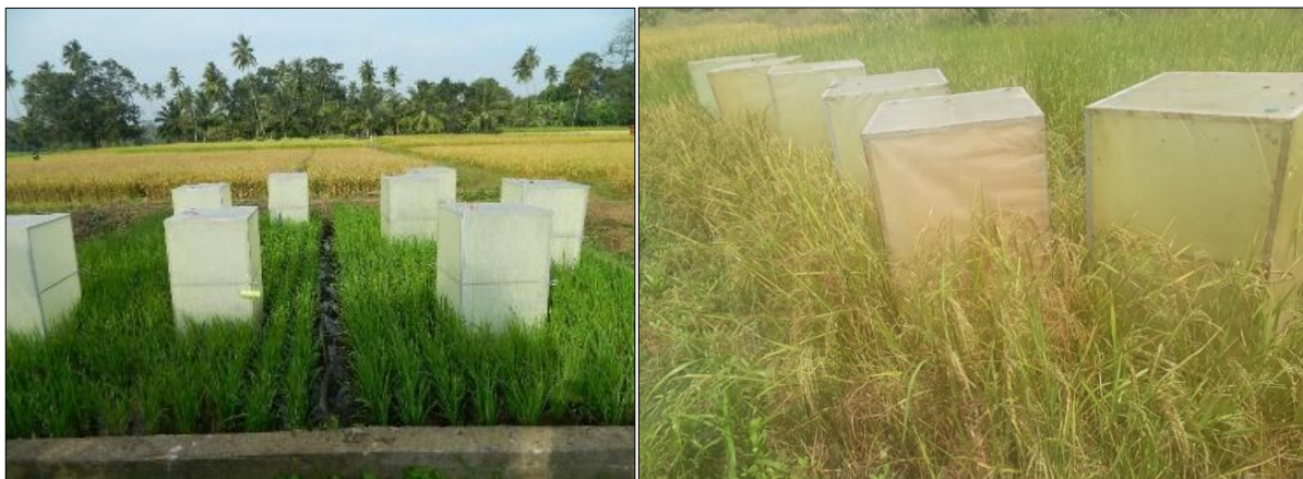
Fig 2: Illustration of chamber used for collection of GHGs from experimental plots
