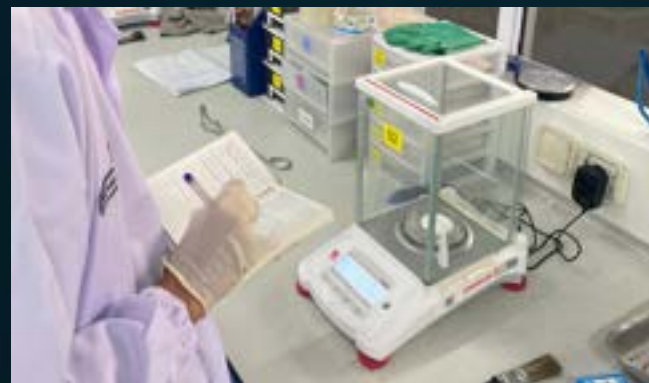
WEIGHING THE INITIAL WEIGHT OF FILTER PAPER & PETRI DISHES
