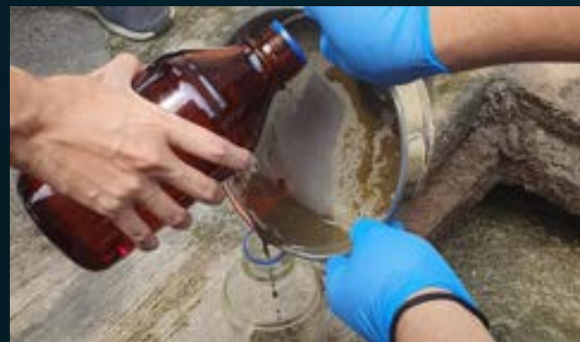
SIEVED SOLIDS TRANSFER
