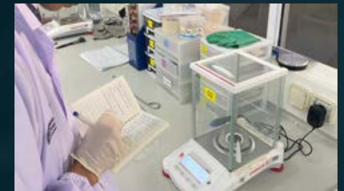
FINAL WEIGHING OF FILTER PAPER AND PETRI DISHES
