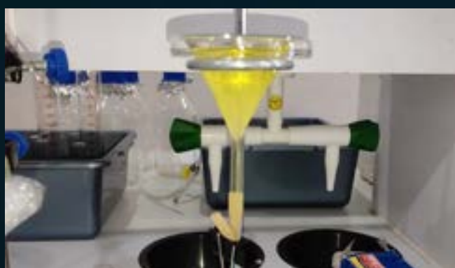
SEPARATION OF SOLIDS IN DENSITY SEPARATOR
