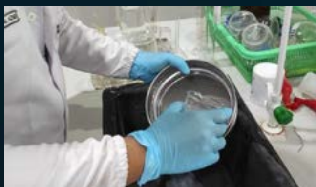
SIEVED SOLIDS TRANSFER
