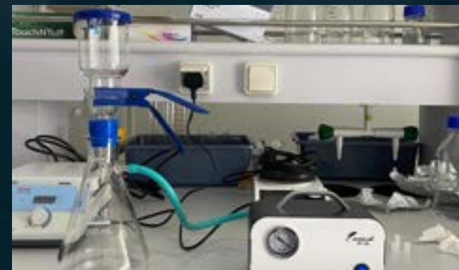
RAINWATER SAMPLE FILTRATION
