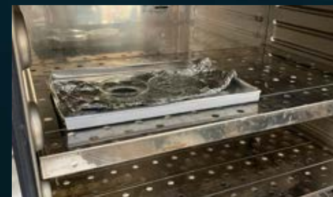
DRYING OF RAINWATER SAMPLES AFTER NILE RED SOLUTION
