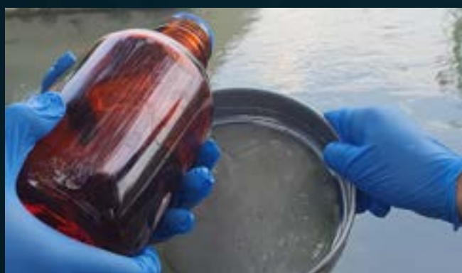
SIEVED SOLIDS TRANSFER
