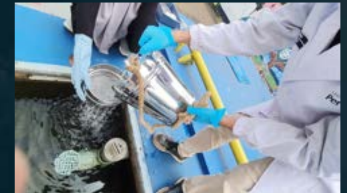
WET SCREENING OF SAMPLES
