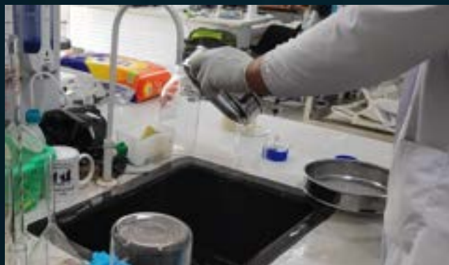
SIEVED SOLIDS TRANSFER
