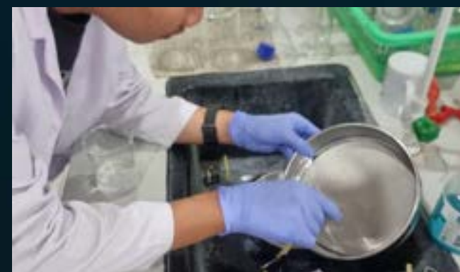
SIEVED SOLIDS TRANSFER
