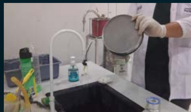
SIEVED SOLIDS TRANSFER
