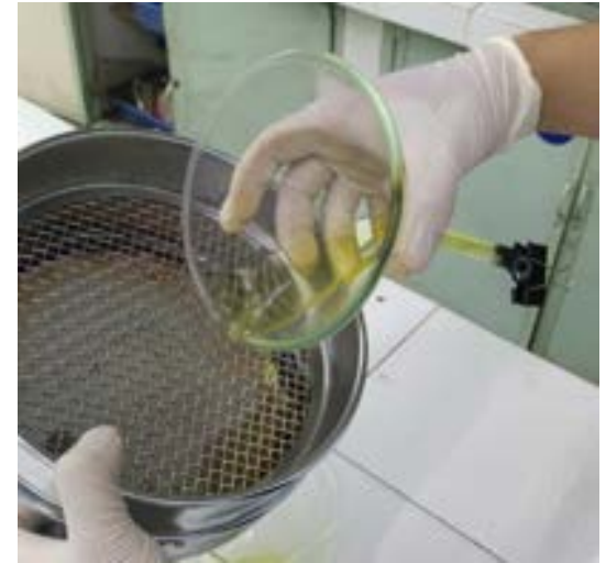
Collect floating solids in a clean 12 \mu\text{m} sieve
