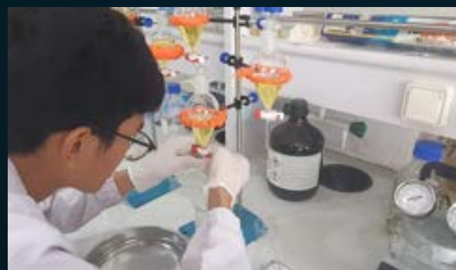
SEPARATION OF SOLIDS IN DENSITY SEPARATOR
