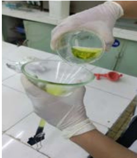
Transfer the WPO solution to the density separator
