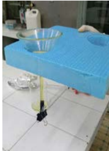
Rinse the WPO beaker with distilled water several times to transfer all remaining solids to the density separator → and allow solids to settle overnight (24 hour)
