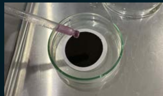
ADDITION OF NILE RED SOLUTION TO FILTER PAPER
