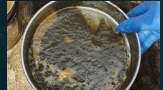
WET SCREENING OF SAMPLES
