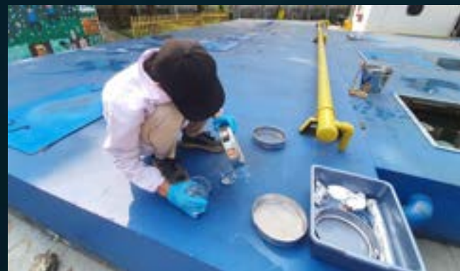
SIEVED SOLIDS TRANSFER
