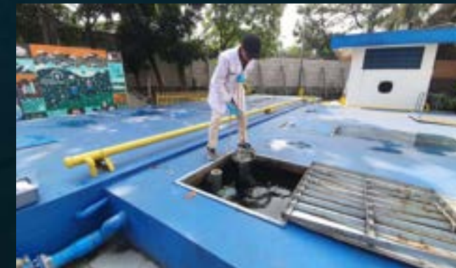
SAMPLING OF WWTP INFLUENT AND EFFLUENT
