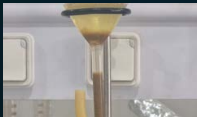
SEPARATION OF SOLIDS IN DENSITY SEPARATOR
