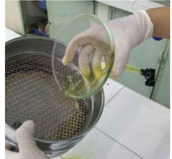
Collect floating solids in a clean 12 µm sieve
