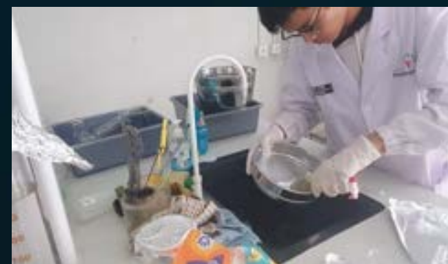
SIEVED SOLIDS TRANSFER
