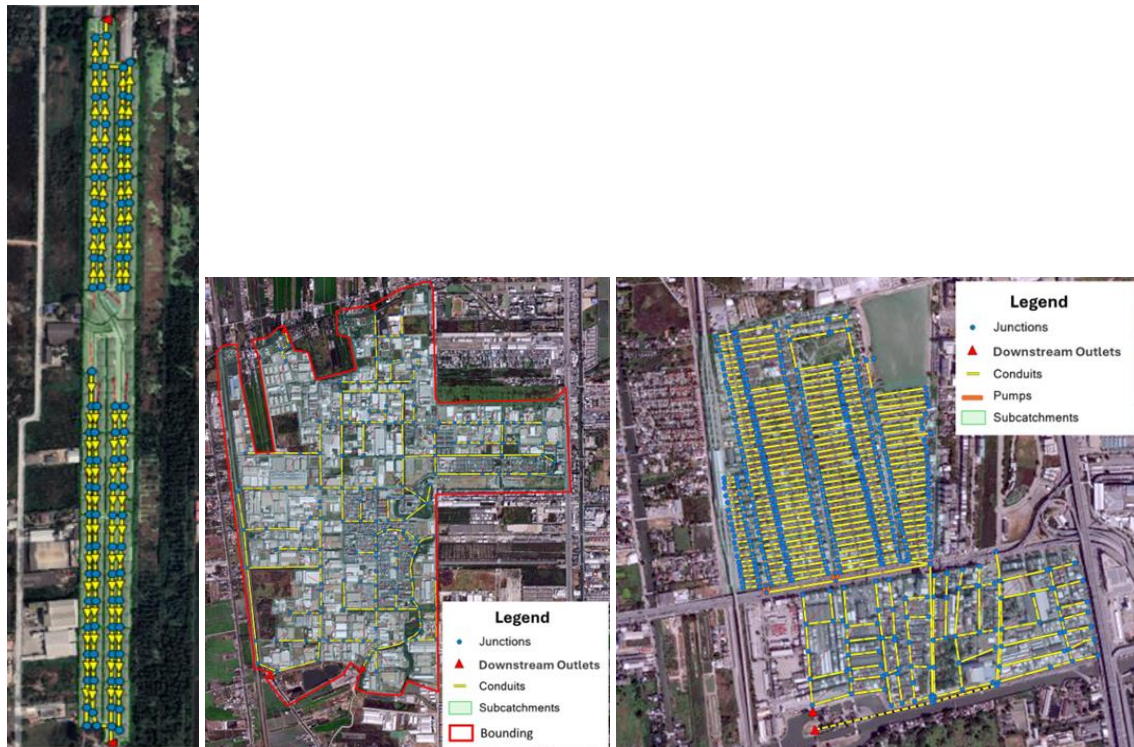
Figure 5 Drainage system components visualized in PCSWMM for selected urbanized areas, moo baan (left); Nava Nakorn industrial estate (middle); and Ratanakosin Village, Rangsit (right).
