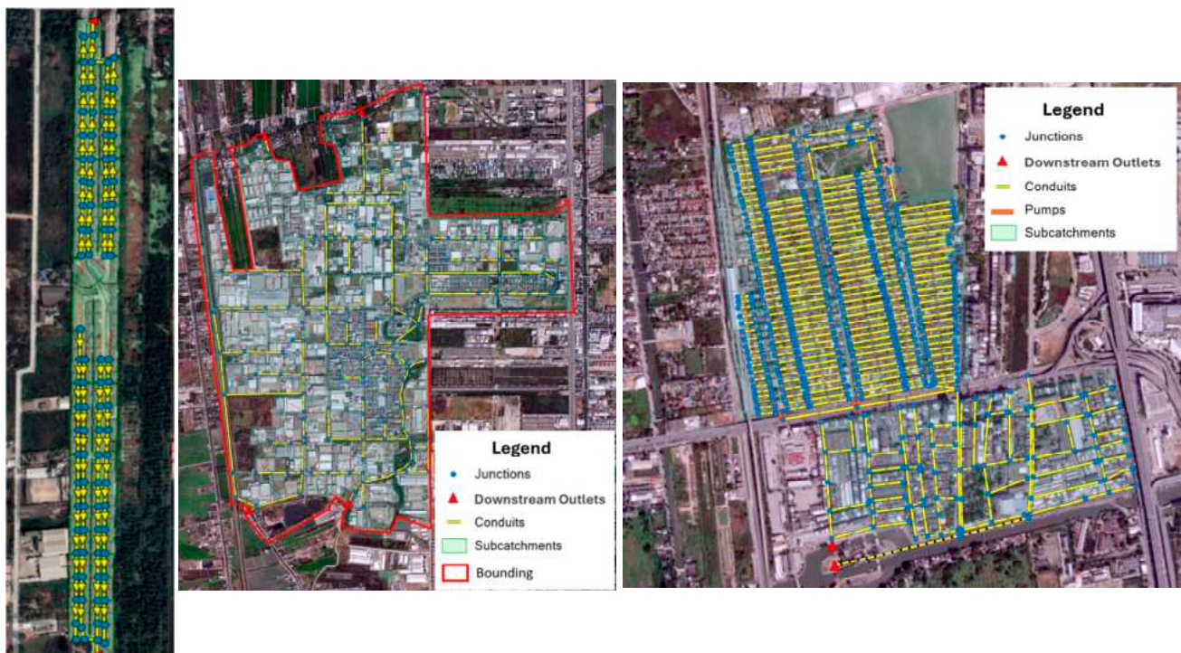
Figure 4. Drainage system components visualized in PCSWMM for selected urbanized areas, moo baan (left); Nava Nakorn industrial estate (middle); and Ratanakosin Village, Rangsit (right). Pump locations are circled in orange for clarity.
