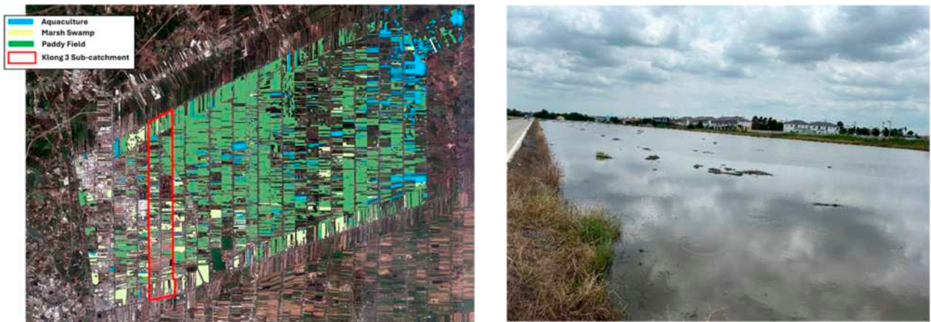
Figure 5. Land use map highlighting paddy fields and surface storage assumptions in the study area (left) and example paddy field storage (right).
