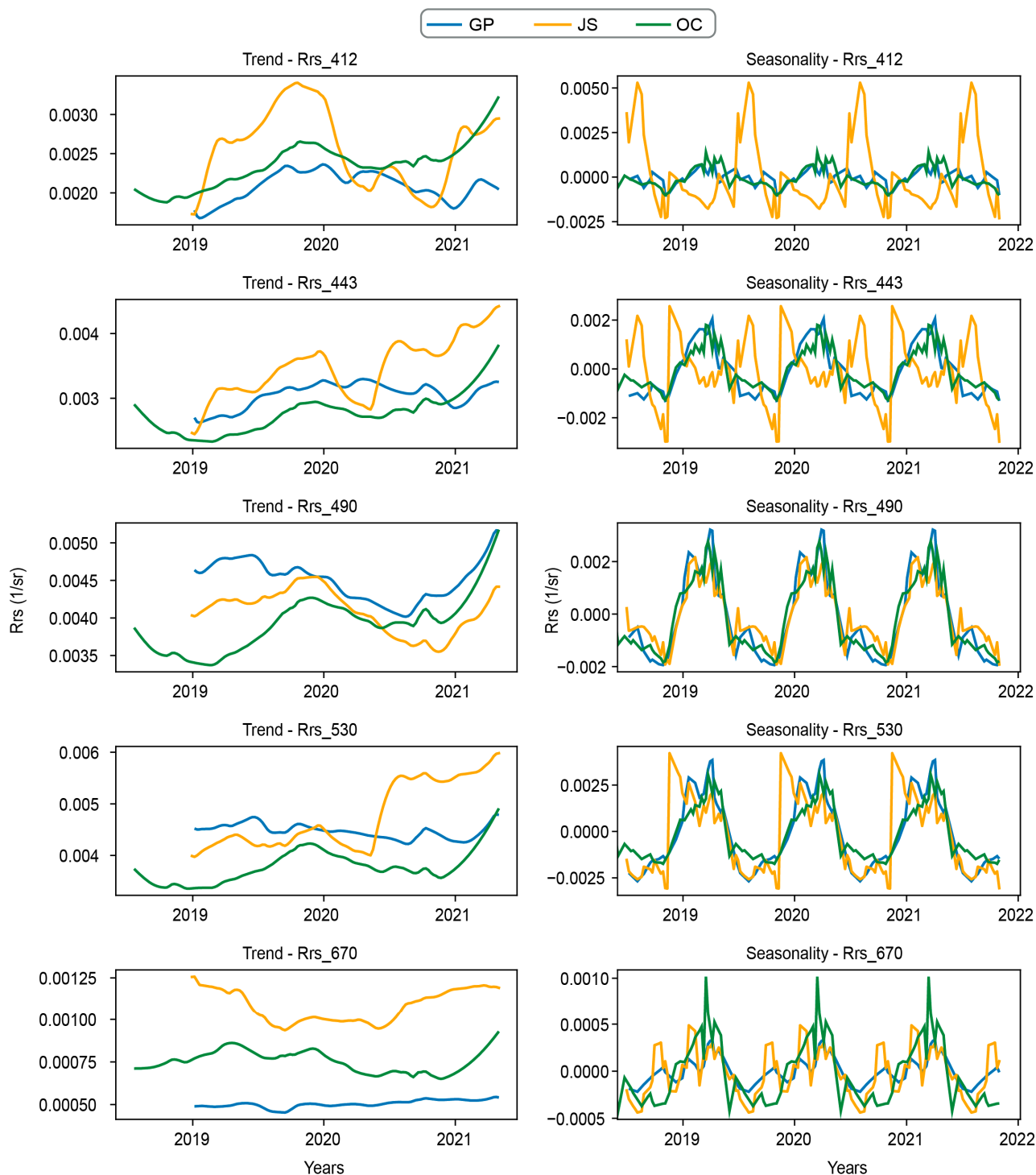
Figure A1. Trend and seasonality components of R_{rs} for five key bands ( R_{rs\_412} , R_{rs\_443} , R_{rs\_490} , R_{rs\_530} , and R_{rs\_670} ) at the Socheongcho AERONET-OC site. The trend plots (left column) and seasonality plots (right column) illustrate the temporal behavior of remote sensing reflectance across G-Portal, JASMES, and AERONET-OC data.
