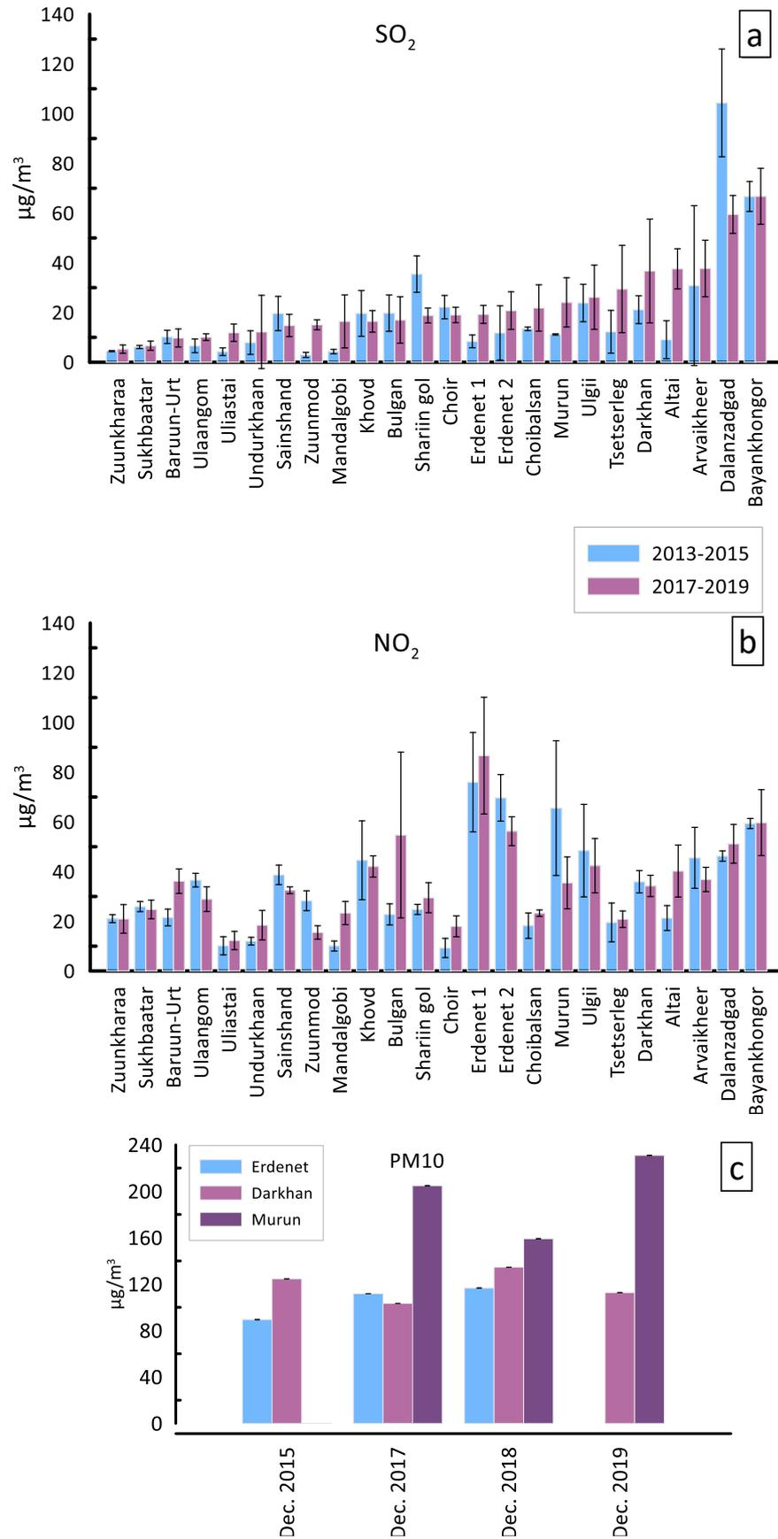
**Fig. 2.** Monthly mean concentrations for December of (a) SO<sub>2</sub>, (b) NO<sub>2</sub>, and (c) PM<sub>10</sub> at the air quality monitoring sites.
