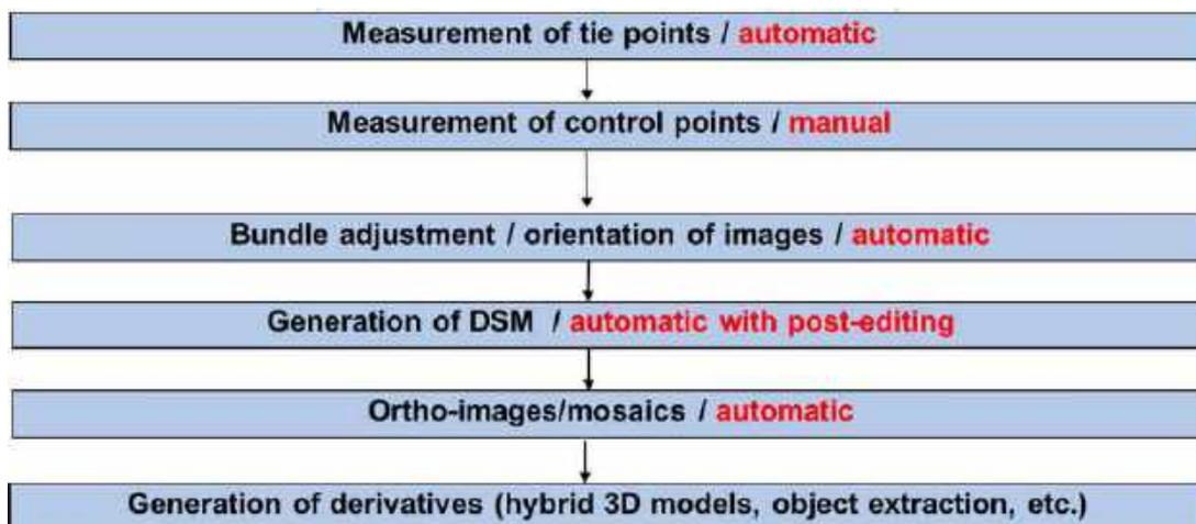
**Figure 9.** The process for deriving drone large scale-map (Qin, 2021)
