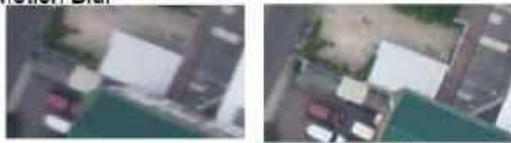
Pixel blur =  $\frac{\text{Ground Speed} \times \text{Exposure Time}}{\text{GSD}}$
