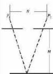
B/H ratio determines the vertical accuracy of the ray resection relative to the horizontal accuracy:
