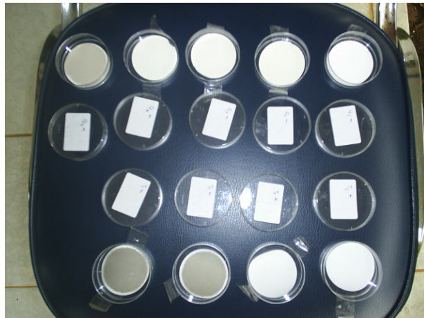
Observation of PM10 total filtration filters for qualitative analysis of the emissions prior to weighing for PM emission load determination
