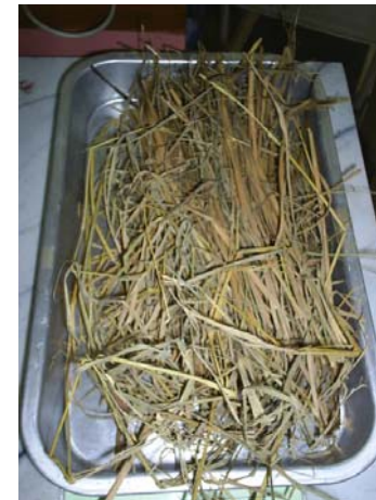
Sample is dried in an oven at 105°C during 24 h for determination of dry weight and moisture content
