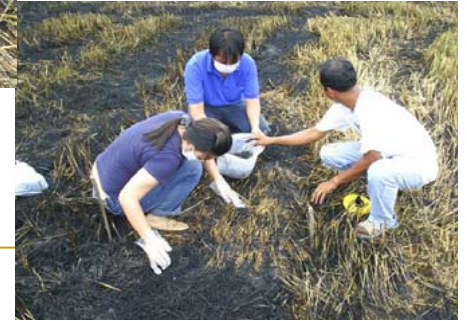
Sampling of ash for the determination of fraction released to the Air
