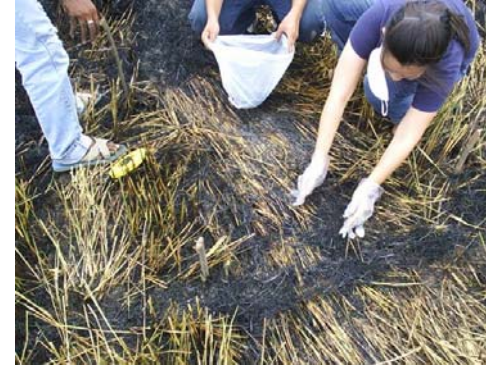
Sampling of unburned biomass for the determination of fraction burned
