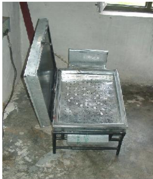
Figure 4. The inner view of a solar dryer used to dry sediment in a filter paper at Narayanghat.
