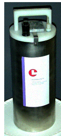
Fig. 3b Recording tide gauge (MicroTide, Coastal Leasing)
