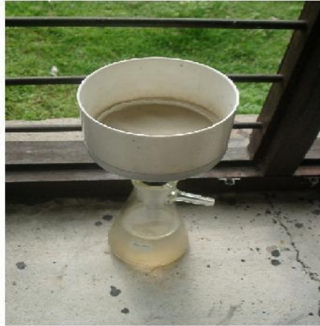
Figure 3. Set-up for a simple system for the filtration of sediment used at Narayanghat. The method uses a Buchner funnel, a pyrex vacuum flask and a filter paper.
