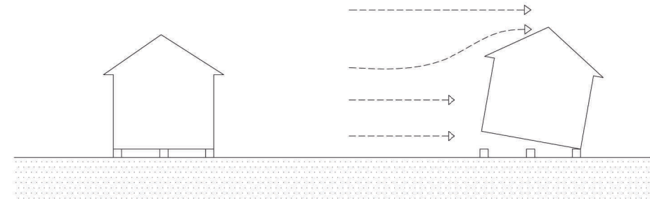
Well-constructed buildings which are not well-anchored down to their foundations may overturn.
