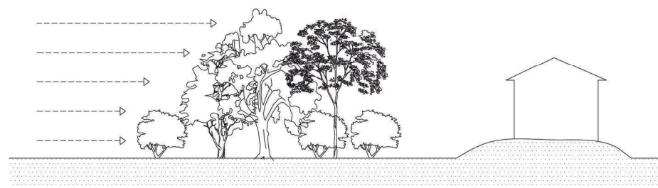
Building shielded by vegetation placed at distance equal to tallest wind-break tree at full growth and built upon raised plinth is well-protected against wind and flood.
