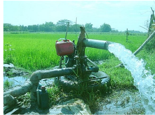
Figure 2. A typical shallow tubewell (STW).
