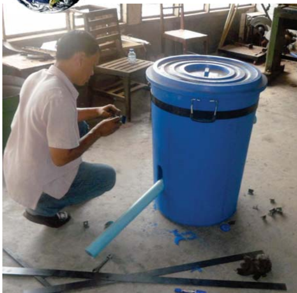
Biogas Tank is Made of plastic water container 168L
