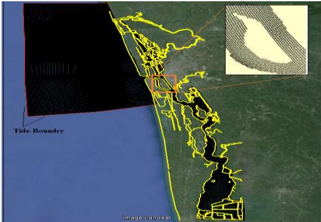
**Figure 55 Grid used for Delft-3D model**
