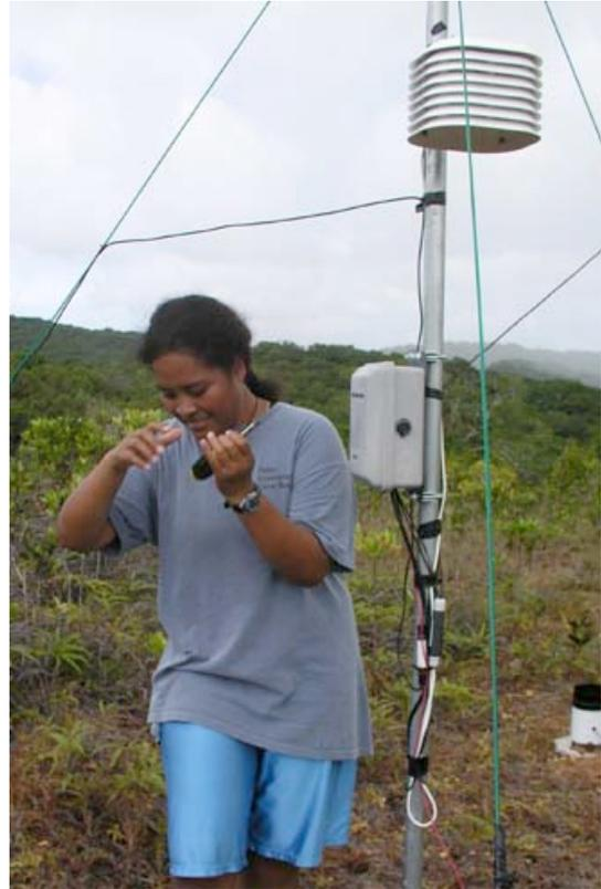
Ms Kimie Ngirchechol preparing to open up the Ngerikiil watershed meteorological station's automated logger to download the data, April 5, 2007. Note the rain gauge near the bottom right of the photograph.
