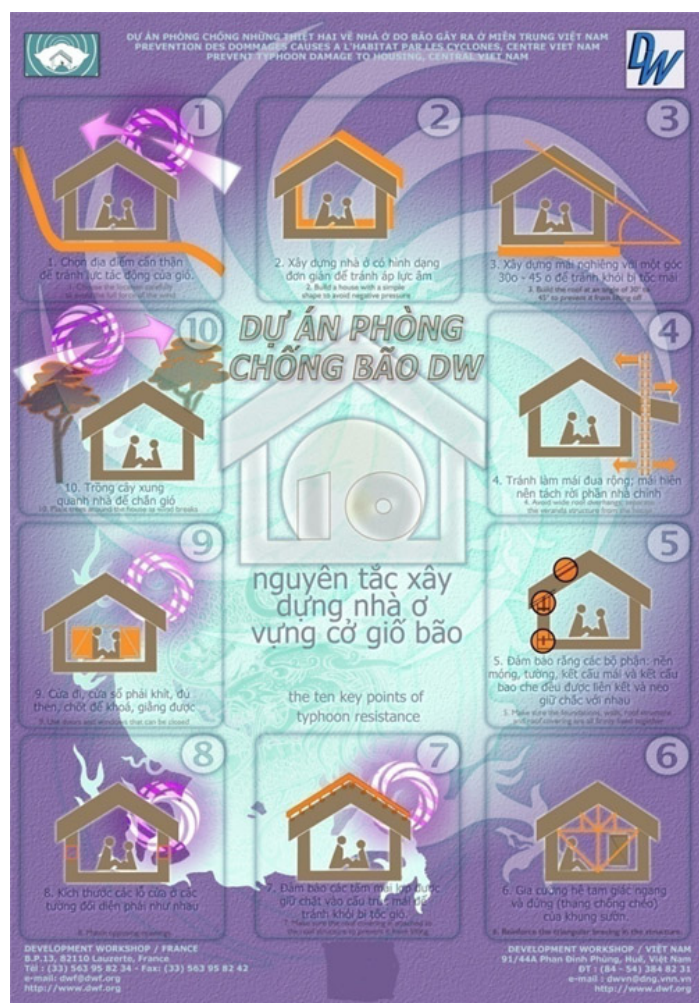
Figure 5: 10 key principles for cyclone-resistant construction (DWF, 2010)
