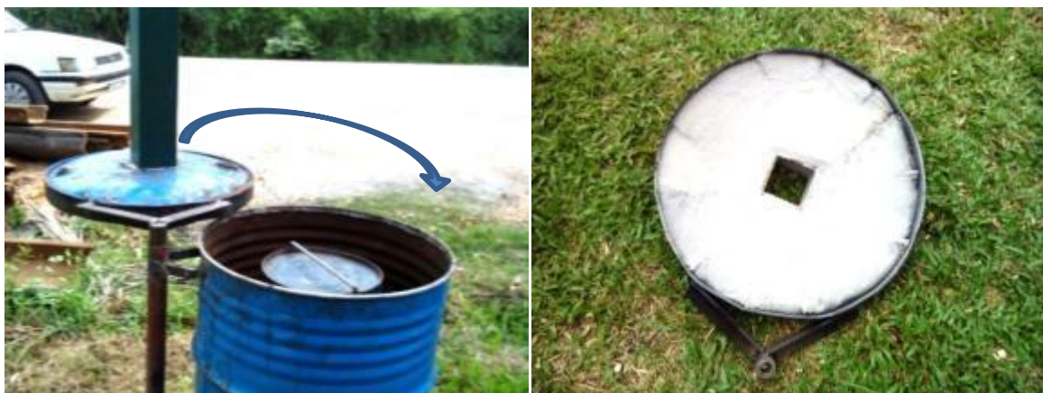
Figure 6: Hinged top lid covered with a layer of refractory material
