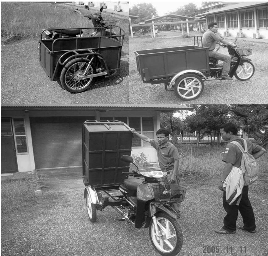
Figure 3.7 Tricycles for waste transportation in the narrow street (Designed and manufactured by University of Lao PDR in 2005)
