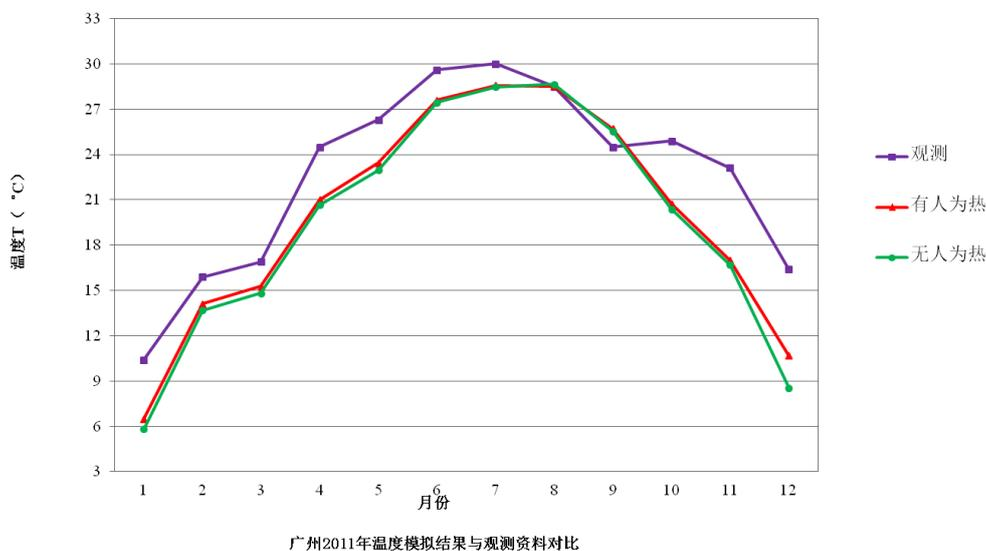
**Figure 25: The simulated and observed surface air temperature of Guangzhou in 2011, units: °C. The blue curve is observation, the green curve is the simulation without anthropogenic heat flux, and the red line is the simulation with anthropogenic heat flux.**
