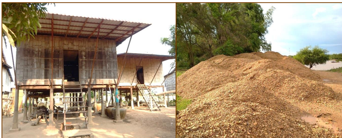
Photos 1 and 2. Common local flooding adaptation measures: extending the stilts of houses (left); building hills for animal evacuation (right)
