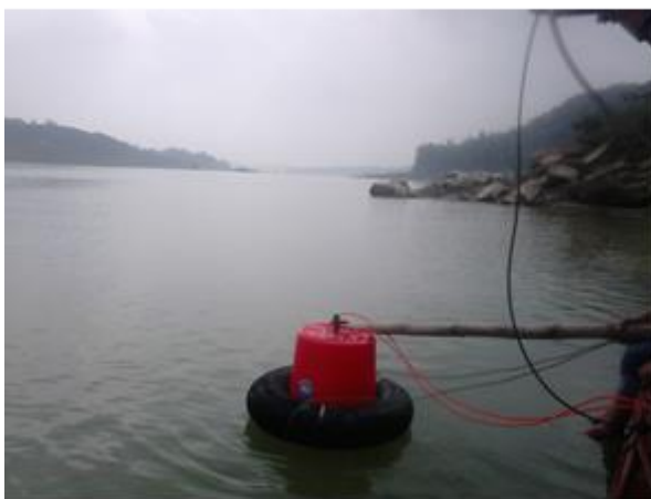
Figure 4. Measurement of carbon exchange at the water-air interface
