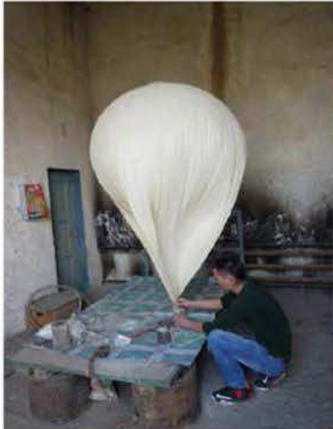
Radiosonde observation. H_2 gas is used.
