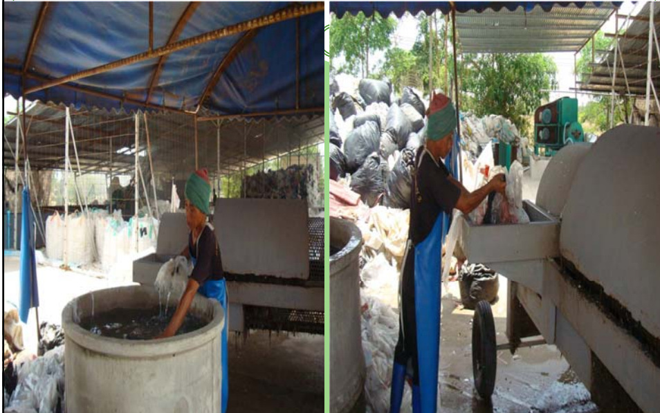
Plastic bag was washed and after that was taken to drum dryer
