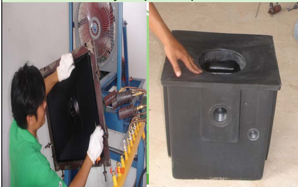
Production of fat trap bucket from recycle plastic powder.
