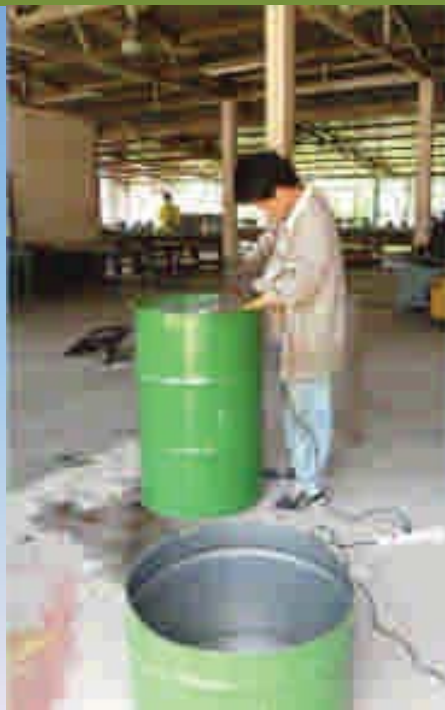
Biogas Tank is made of used steel tank 260L
