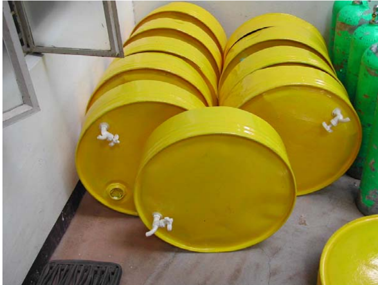
Figure 5 Manual seepage meters prepared at NIGS-UP (National Institute of Geological Sciences, University of The Philippines) specifically for this study.
