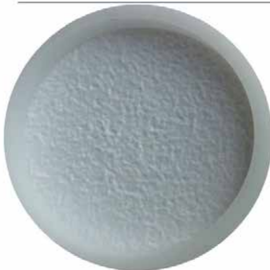
Filter used for PM10 sampling, 16 L/min., Bode, Kathmandu (SusKat-ABC Supersite)
