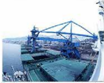
Enclosed continuous unloaders (coal unloader)
