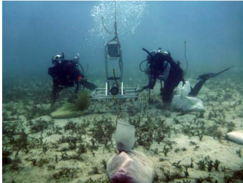
Fig. 3. DIDSON deployed at depth and left for at least 12 hr. to capture dugong images
