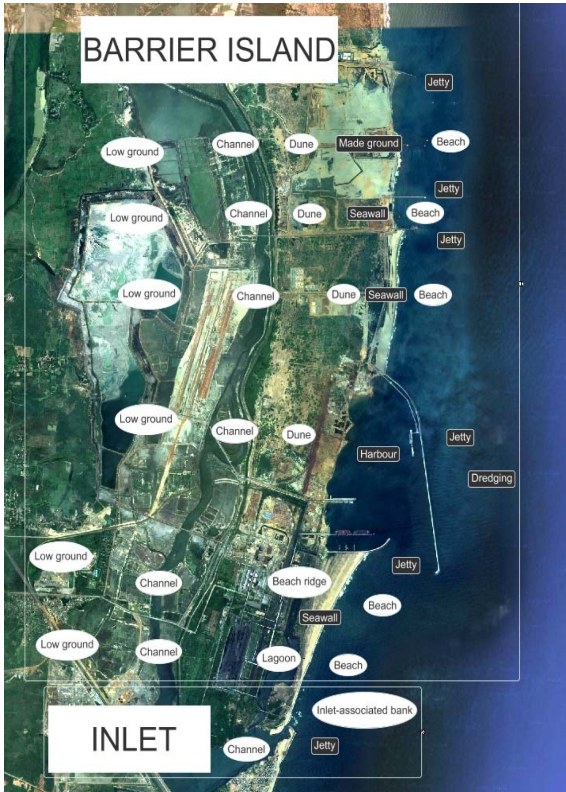
Figure 38 Element groups for inlet and barrier island features.
