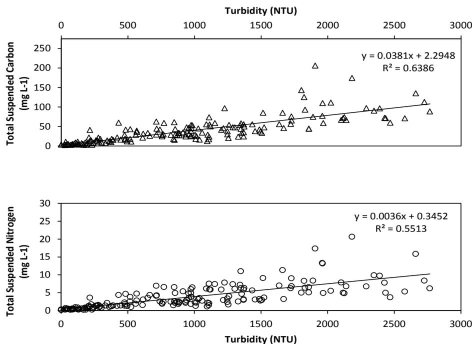
**Figure 12. Linear regression provided a reasonable prediction of total suspended carbon and nitrogen from automated turbidity measurements (From Benner et al., submitted).**
