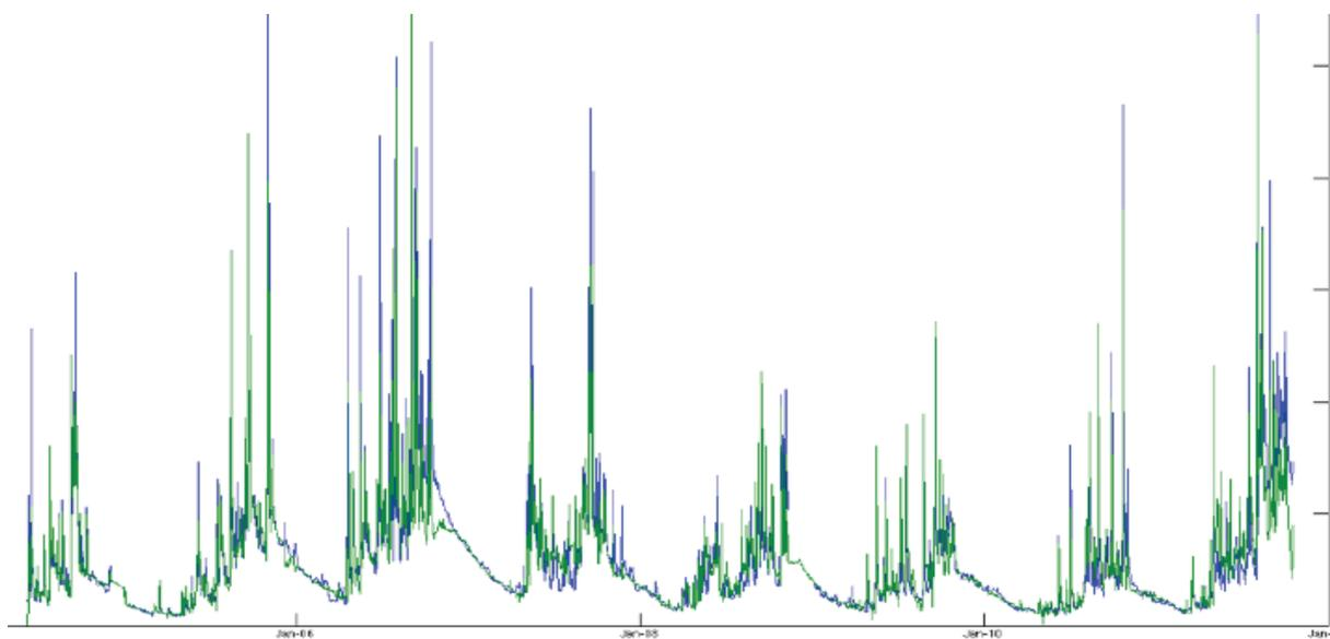
**Figure 17. Observed daily and predicted stream flow in the Mae Sa River (Thailand) for the period 2006-2010. Streamflow is predicted with a support vector machine using the spatial distribution of rainfall (measured at 11 locations), and stream flow from the previous time stamp. Model efficiency was 0.83 for the 8 year simulation.**
