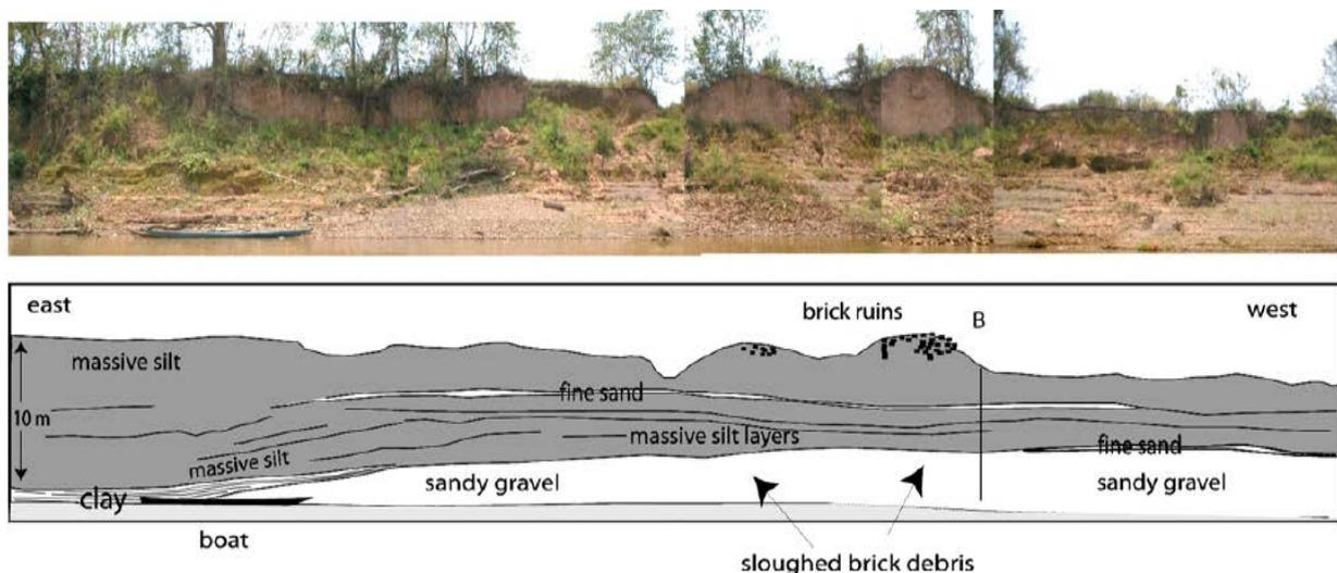
**Figure 18. Cross section view of the floodplain stratigraphy of the Ping River near Chiang Khong Thailand. Alternating layers of silt and sand deposits indicate the occurrence of several large floods, some of which lead to the abandonment of large cities and cause avulsions on some river stretches (From Wood et al., 2008).**
