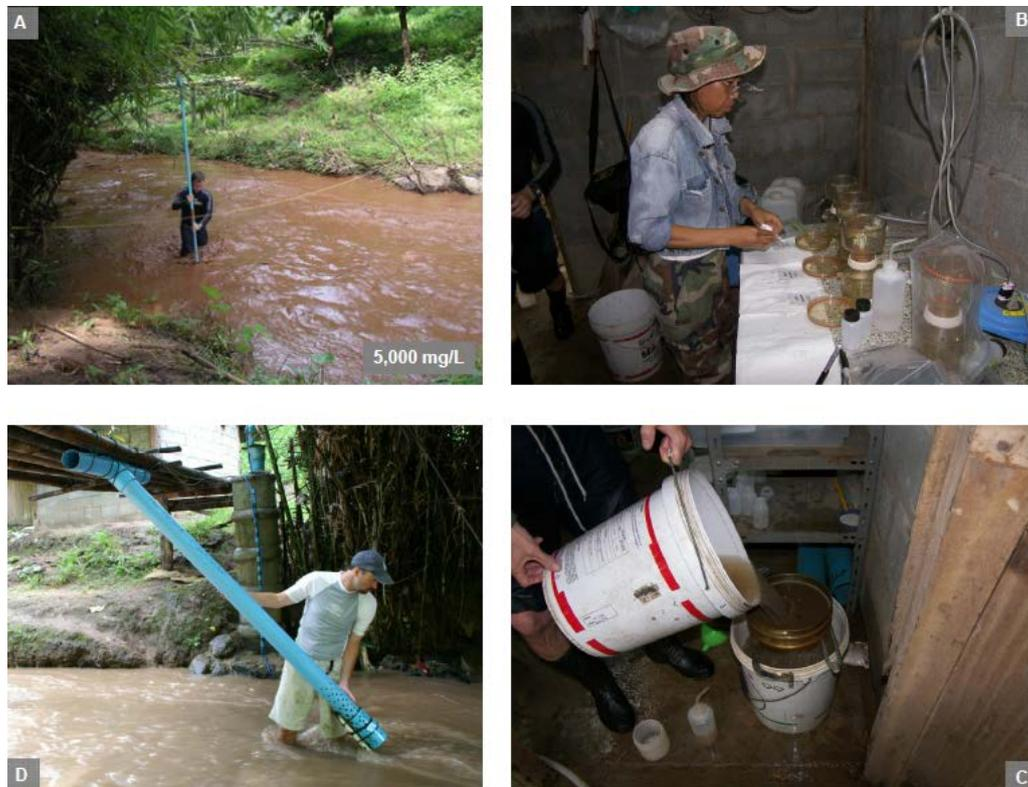
**Figure 5. River sampling in MSEC. (A) Collection of high concentration sediment with depth-integrated sampler; (B) Filtering samples through 0.7um filters; (C) wet sieving large fractions in 20-l samples; and (D) automated turbidity probe installed in cantilever suspended from the bridge (From Ziegler et al., submitted).**
