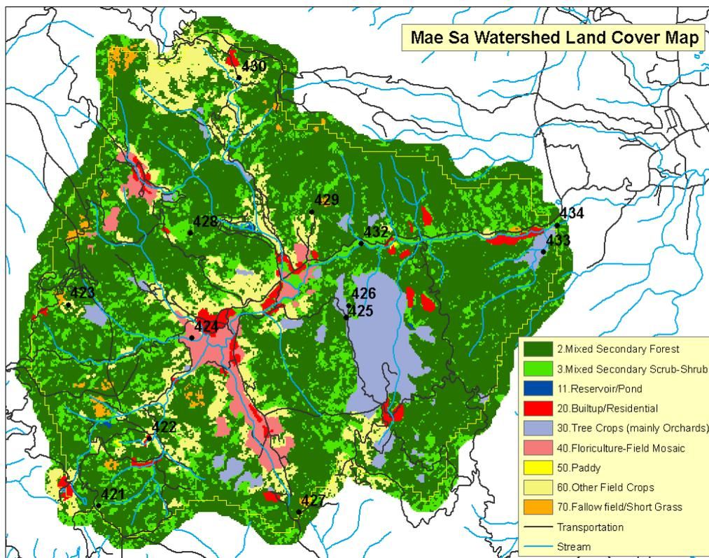
**Fig. 4** Mae Sa Experimental Catchment (MSEC) study area in northern Thailand (see Figure 1,3). Streamflow is monitored at one location (434); energy flux variables for estimating evapotranspiration at three locations (421, 429, 433); soil moisture at six locations (421, 423, 425, 428, 429, 433); and rainfall at eleven locations (all but 425 and 434). Adapted from Ziegler et al (submitted).
