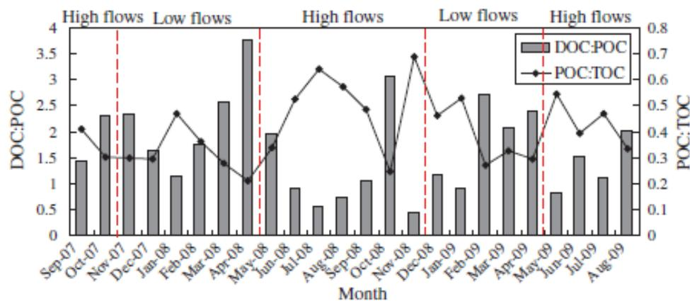
**Figure 13: Seasonal changes DOC, POC, and TOC relationships. TOC was largely regulated by POC in the high flow period but by DOC in the low flow period, which was consistent with higher POC/TOC ratio occurred in the high flow period but higher DOC/TOC ratio in the low flow period (From Lu et al., 2012).**
