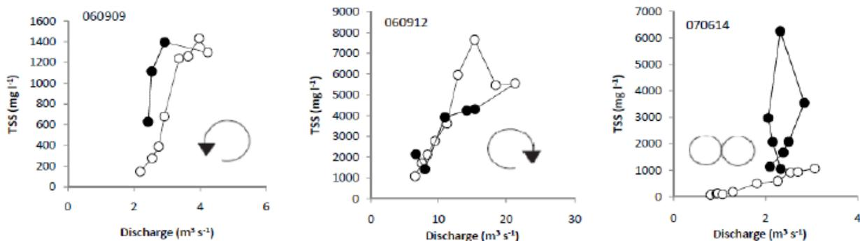
**Figure 10.** Various types of hysteresis in the discharge-TSS (total suspended solids) relationship were observed: anti-clockwise, clockwise, and figure eight, respectively (left to right). Labels refer to sampling dates (From Ziegler et al., submitted).
