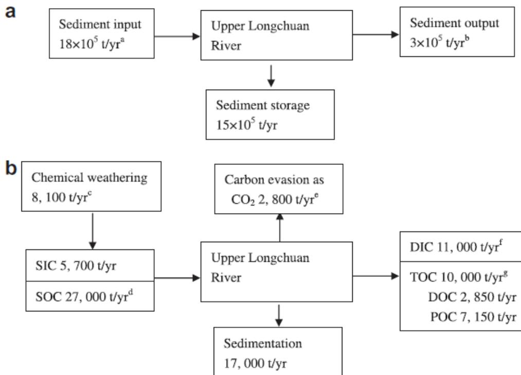
Figure 14. Sediment (a) and carbon (b) budgets for the upper Longchuang River (Li et al, forthcoming). SOC and SIC, refer to soil organic and inorganic carbon.
