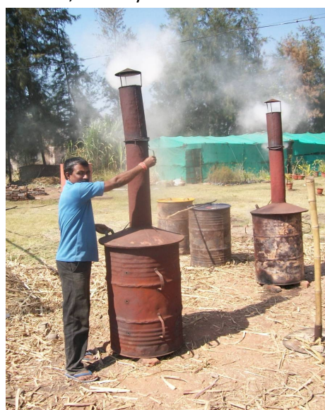
FIGURE 17: ARTI'S SINGLE BARRLE KILNS IN OPERATION. FEEDSTOCK USED: SUGARCANE TRASH
