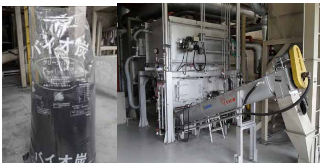
FIGURE 34: CARBONISED RICE HUSKS FOR SALE IN 30KG SACKS IN JAPAN (LEFT) AND THE CARBONISER WITH MAKES THEM (RIGHT) (COURTESY OF MAŠEK ET AL., 2010).
