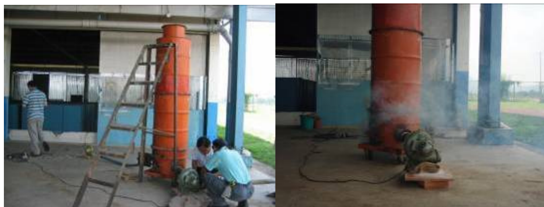
FIGURES 14 AND 15: PREPARATION OF THE GASIFIER AND INITIAL HEATING UP PHASE. THE GASIFIER CHAMBER WAS SITUATED IN THE SECOND BARREL FROM THE BOTTOM AND HAD AN INNER DIAMETER OF 0.46 M, A HEIGHT OF 0.97 M, AND A VOLUME OF 161.2 LITER.
