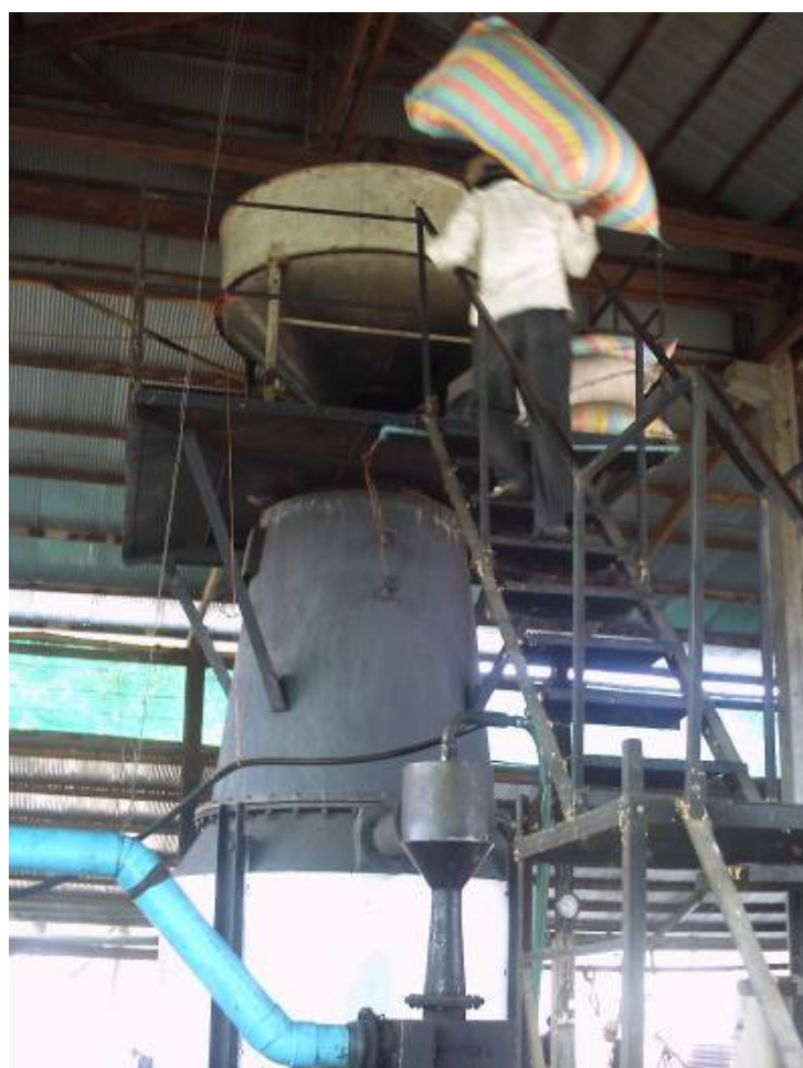
FIGURE 4: RICE HUSKS BEING LOADED INTO AN ANKUR GASIFIER NEAR SIEM REAP, CAMBODIA
