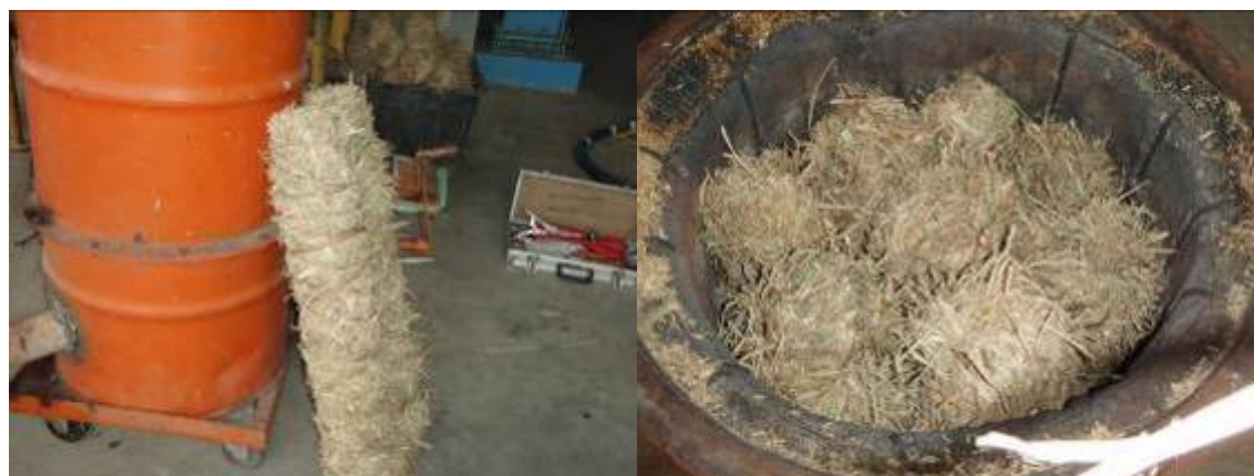
FIGURE 16: WE USED TIGHTLY BUNDLED STRAW IN THE SECOND ATTEMPT FOR STRAW GASIFICATION BECAUSE WE ASSUMED THAT THE LOW FUEL DENSITY WAS THE REASON FOR THE POOR GASIFICATION.
