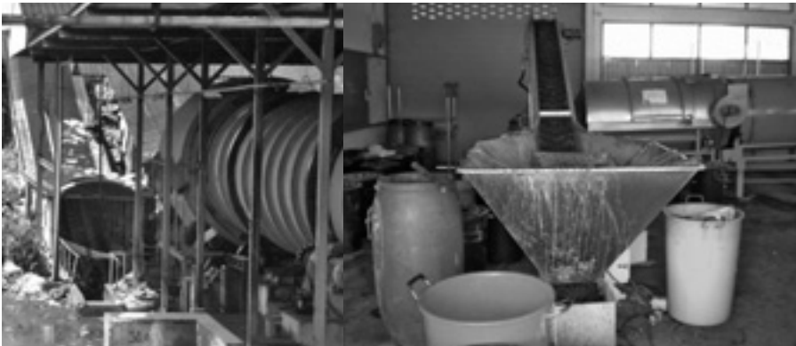
Figure 3.12 In-vessel composting in Thailand
