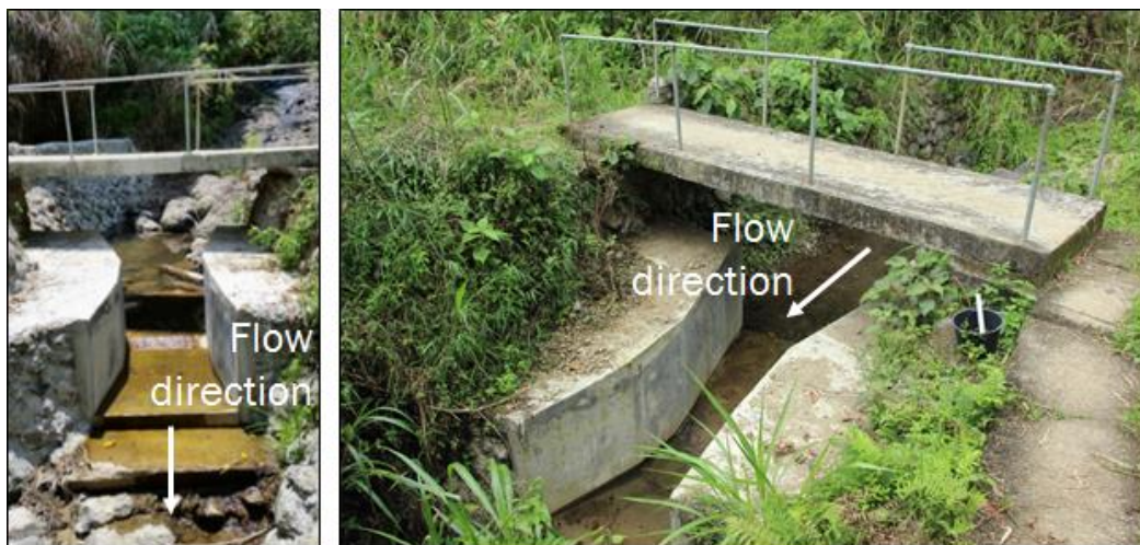
Figure 14. Parshall Flume installed in the selected terrace catchment for the measurement of stream flow.
