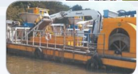
A Conveyor Boat Size 6x14 m
