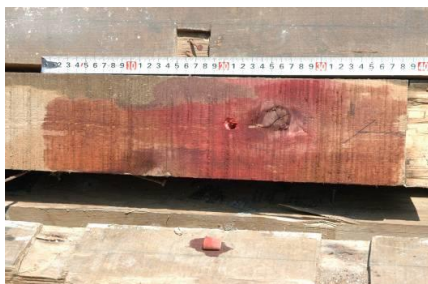
Checking for CCA-treated wood using a reagent
