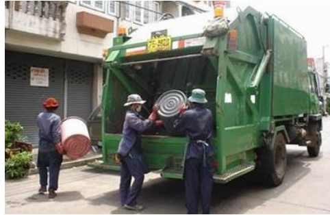
Figure 2.2 Manually loaded waste truck
