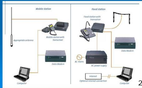
Typical HF radio Email system set-up
