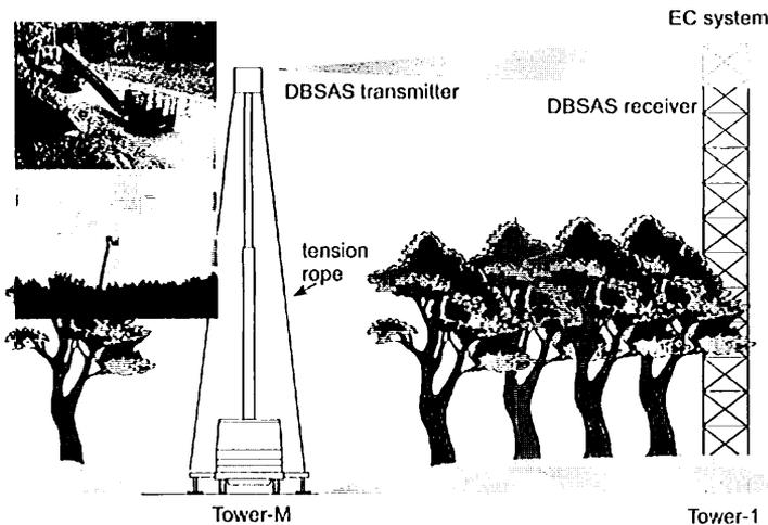
Fig 2. Mobile elevated work platform as an additional tower for the DBSAS
