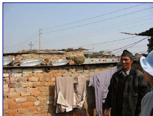
Figure: SODIS: PET bottles on the roof
