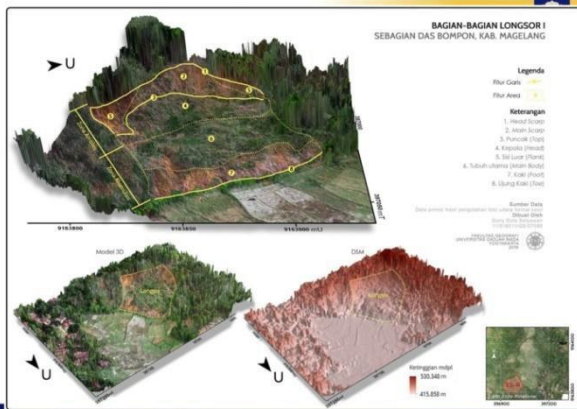
DEM modeled from DSM
