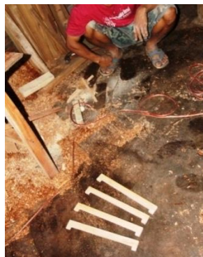
Photo 16: Local manufacture of Christen hypsometer
