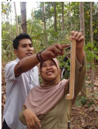
Photo 15: ARuPA forester instructing female village leader on the use of a Christen hypsometer
