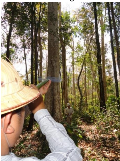
Photo 14: Estimating tree diameter above buttresses using “locally appropriate” technology
