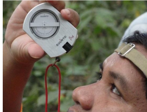
Photo 7: Using SUUNTO to estimate tree height, Seima, Cambodia
