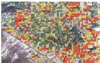
IEWS damage assessment: Texture-based change detection
