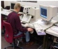
Manual measurements on analogue stereo images with an analytical plotter
