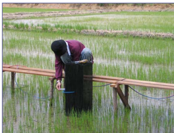
Above: Setting up of field experimental procedures in paddy fields for measuring emissions from biogenic sources
